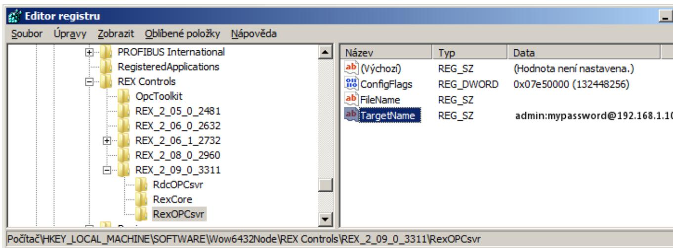
Afterwards it is possible to establish data exchange with the running executive of the REXYGEN system from the visualization software. The OPC server named `REXControls.REX OPCsvr` allows the visualization SW to read all inputs, outputs and parameters of the function blocks the control algorithm is composed of. It is possible to write to function block parameters and inputs. For the latter case, no signal can be connected to the block input in the control algorithm.
