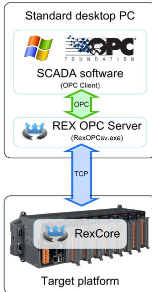
It is necessary to define the IP address of the REXYGEN target device in Windows registry to allow data exchange with the OPC server. Find the following key in the Windows registry
