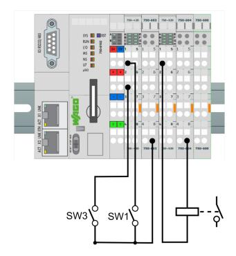
IMPORTANT: Note that numbering of the terminals on the WAGO modules (above) does not comply with channel numbering (below)! Always follow the DI1..8, DO1..8, AI1..4, etc. notation as per WAGO documentation.
