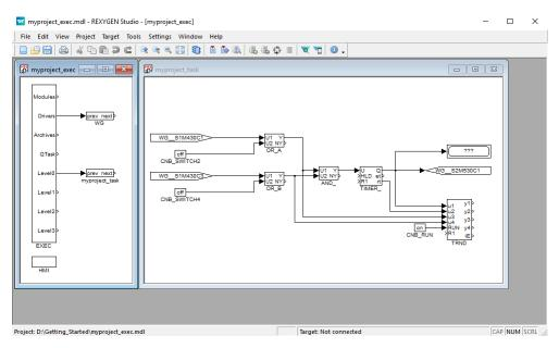
After compiling the project and downloading it to the WAGO PFC100/200 the control algorithm interacts with the physical world. Again it is possible to switch to Watch mode and observe the signals in real-time or analyze the trends of signals. Flip the physical switches and watch the signals.
