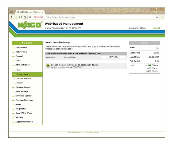
7. Power-off the Wago PLC, remove the SD card and power it on again.
