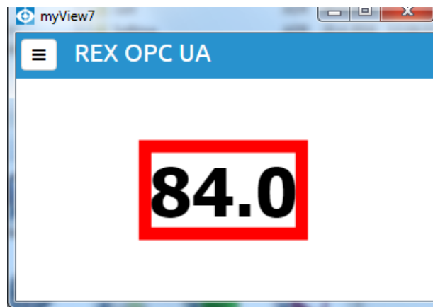
Figure 7.22: mySCADA: Data tag is not available
