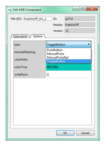
Now we have four PushOnOff buttons and one Display and we want to link all components with live data from the target device.
