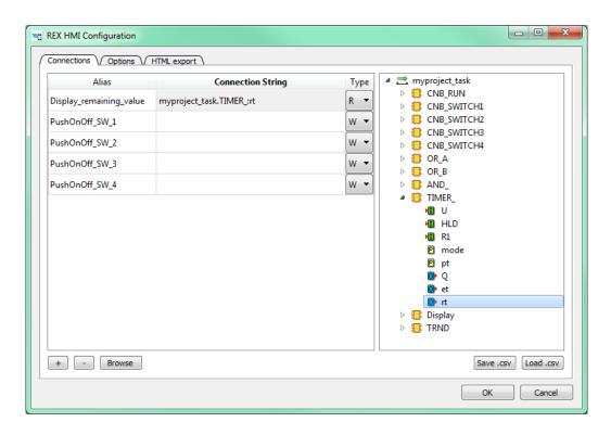
Once the display is linked we will also link the switches. Just browse the tree to CNB\_SWITCH1, select the *Connection String* field of the *PushOnOff\_SW\_1* alias and double-click the YCN parameter. Repeat this for the remaining connection strings. Afterwards press OK to save the settings and close the dialog.
