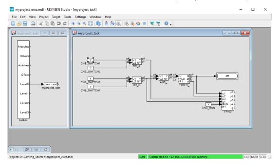
Now it is possible to double-click the CNB\_SWITCH1 block and change the Boolean variable to YCN = on (tick the checkbox and click OK). Once you do the same with the CNB\_SWITCH3 block, the outputs of both OR blocks are on and the Y output of the AND\_ block goes on and the TIMER\_ starts to count down. Observe the rt output.<sup>2</sup> Once the
