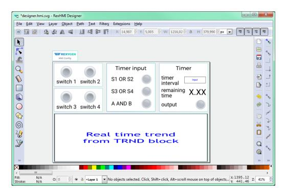
As mentioned earlier, the \*.hmi.svg files in the hmisrc folder are automatically processed while the project is compiled in the REXYGEN Studio application. The project main file must contain the HMI block with GenerateRexHMI parameter enabled. This was already covered in Section 6.3 so you should have everything ready.
