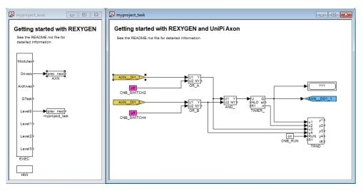
After compiling the project and downloading it to the UniPi Axon/Patron the control algorithm interacts with the physical world. Again it is possible to switch to Watch mode and observe the signals in real-time or analyze the trends of signals. Flip the physical switches and watch the signals.
