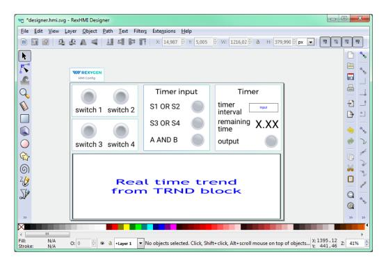
As mentioned earlier, the \*.hmi.svg files in the hmisrc folder are automatically processed while the project is compiled in the REXYGEN Studio application. The project main file must contain the HMI block with GenerateRexHMI parameter enabled. This was already covered in Section 4.3 so you should have everything ready.
