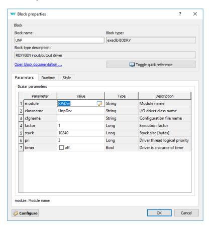
As the final step, rename the  ${\tt IODRV}$  block to UNP, which will serve as a prefix for all  ${\rm I/O}$  signals of this driver.
