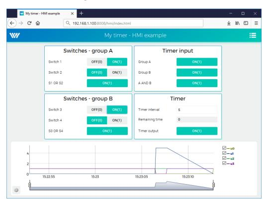
6. You can toggle the switches and observe the results. The virtual switches are linked
