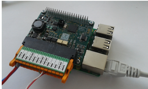
Figure 3.2: Terminal pinout for Monarco HAT.
