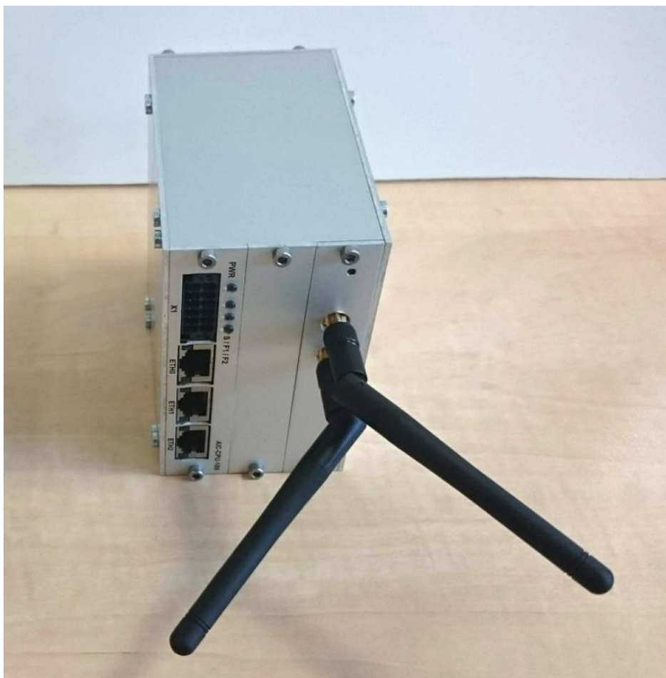
AIC (Advanced Industrial Controller) equipped with RETIS RF plug-in card.
