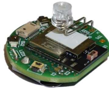
Remotely controlled active motion capture marker for differential motion capture applications. Left - final solution, right - unboxed board.
